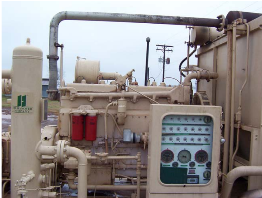
Figure 2-3. Small, uncontrolled, rich-burn compressor engine (Northeast Texas).
